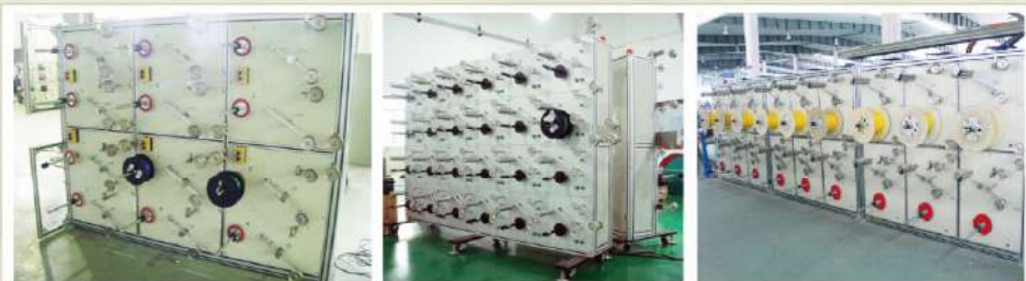
各类光纤、紧包光纤、单芯缆主动放线架 Different kinds of fiber pay-off, buffer and fiber microtube pay-off
