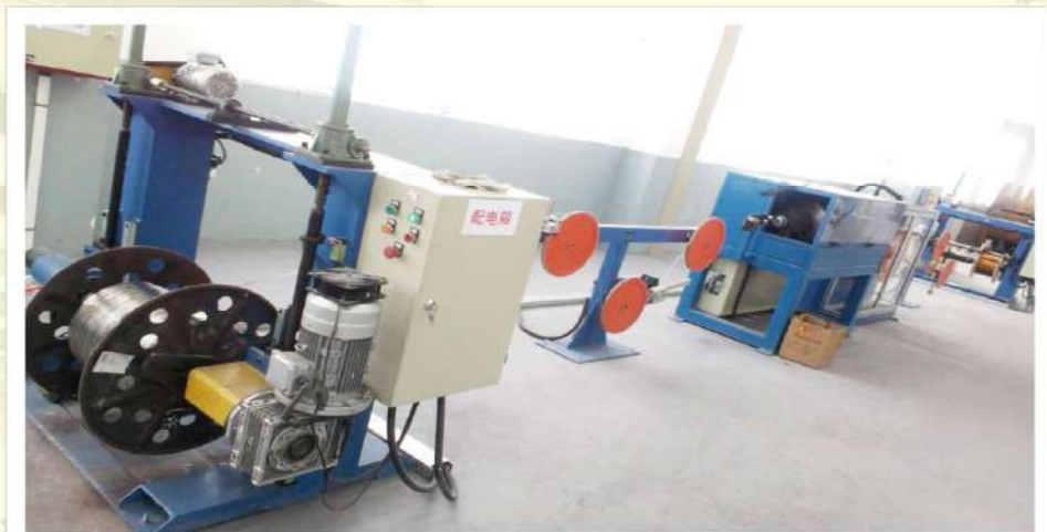
主要用于圆形或扁平的金属导体的绝缘绕包 It is mainly used for insulation taping of round and flat metal conductor
