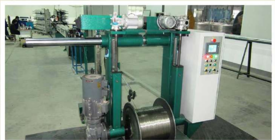
用于生产光纤复合不锈钢管，应用于OPGW，特种缆，海缆上面 Used for making Fibers in steel tube, which is broadly applied in OPGW, Tactical cable, Submarine cable etc.
